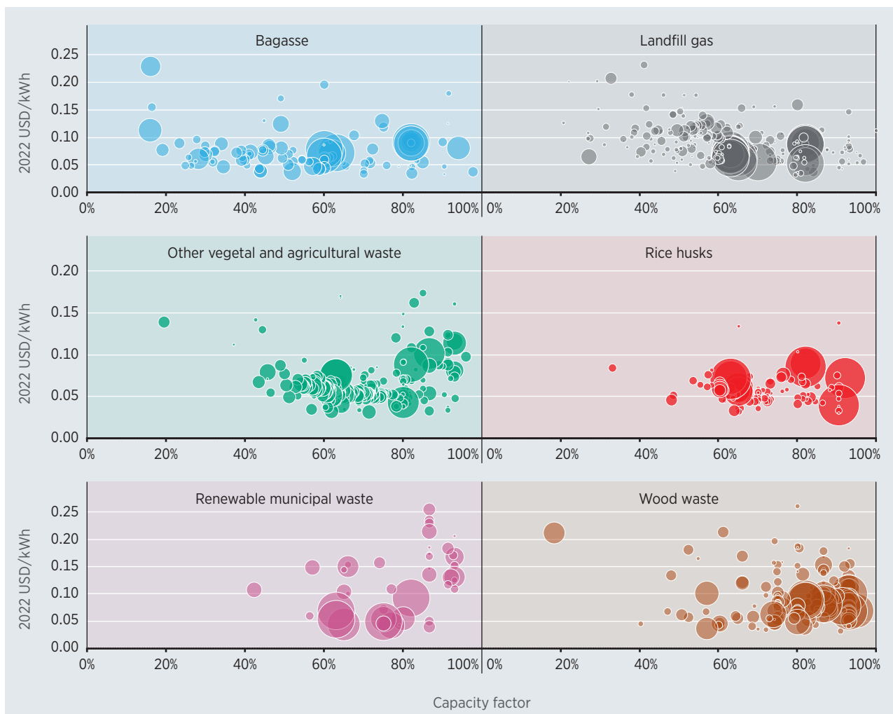
Figure 8.6 LCOE and capacity factor by project of selected feedstocks for bioenergy power generation projects, 2000-2022
