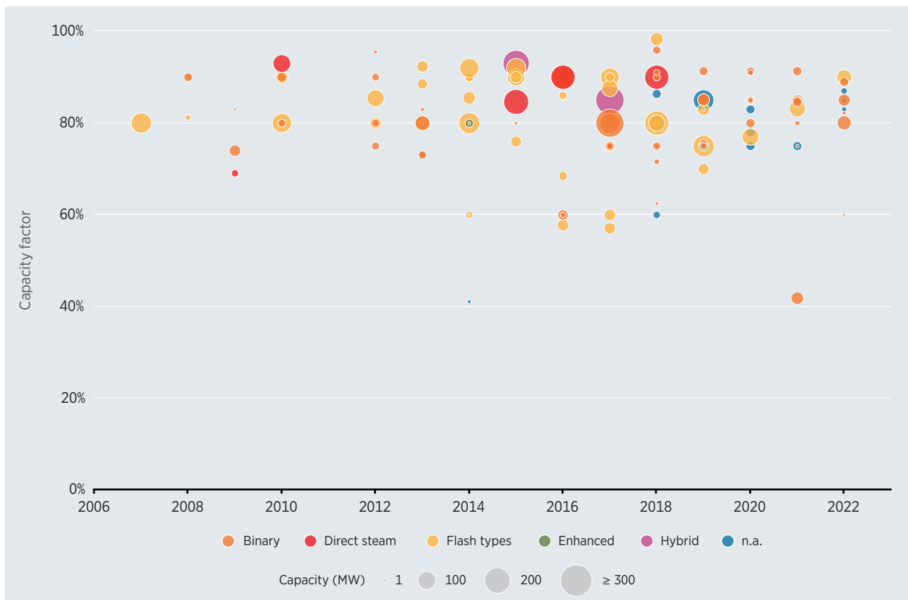
Figure 7.3 Capacity factors of geothermal power plants by technology and project size, 2007-2022
