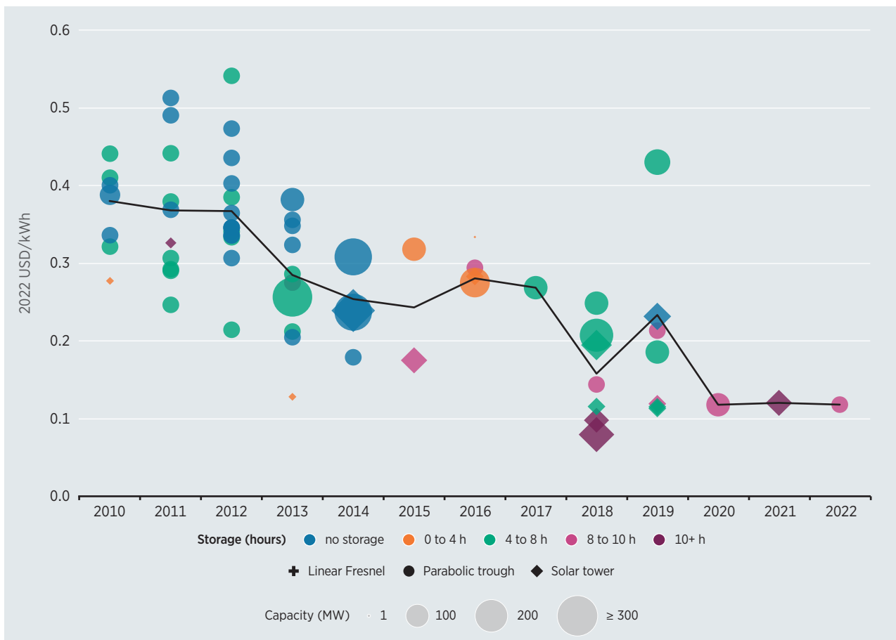
Figure 5.7 LCOE for CSP projects by technology and storage duration, 2010-2022
